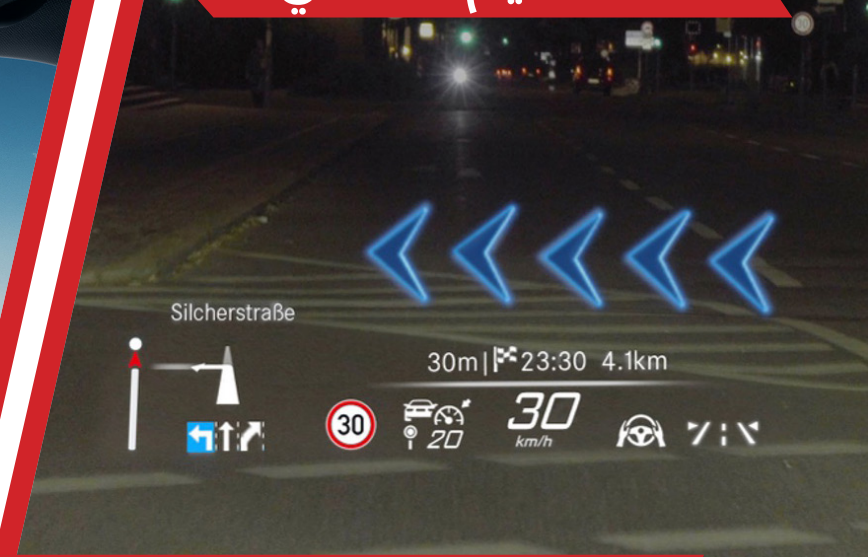
Augmented Reality Head Up Display (HUD)
